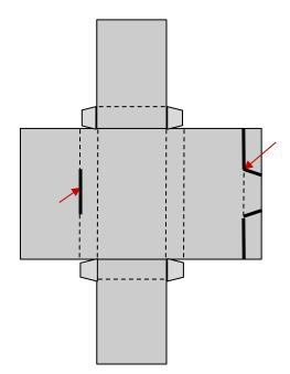
Cut the slot and cut out the tab. The slot should be 2mm wider than the width of the tab.
